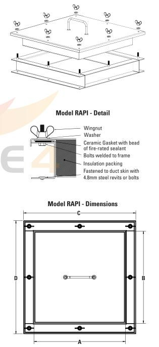
Size of the door shall be A or B + 80mm Size of the frame shall be C or D in mm
