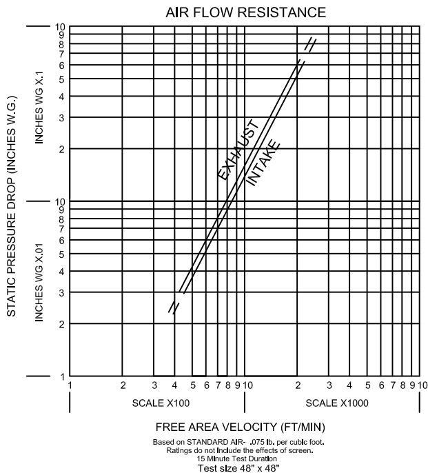
Model SAFL-4 resistance to airflow varies depending on louver application (air intake or air exhaust). Free area velocities (shown) are higher than average velocity through the overall louver size. See louver selection information.
