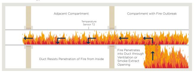
Flamebar BW11 system is tested for up to 4 hours Stability, Integrity and Insulation in accordance with BS 476: Part 24 and ISO 6944 for both Type A and B fires.
