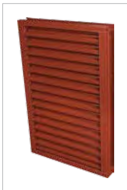
FL-D-2 2" deep, fixed blade, drainable, extruded aluminum
