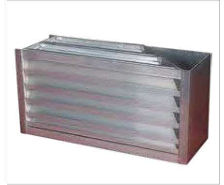
RD-8 8" deep, fixed blade, drainable, wind/rain/sand, extruded aluminum
