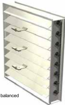
Precision Counter Balanced; both by rotation in hub or slide weight up or down the rod in addition to removal or adding weights.
